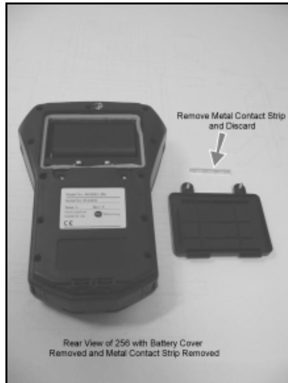
Figure 2 - Metal Contact Strip Removed from Battery Cover
