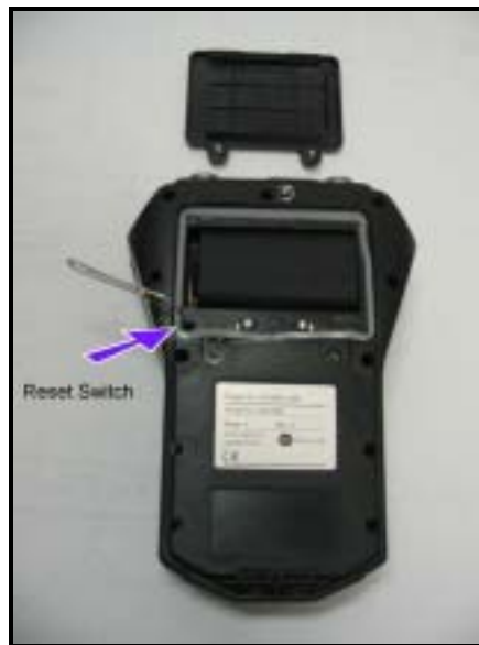
Figure 1 - Rear of 256 with Battery Cover Open with Paper Clip in Reset Switch
