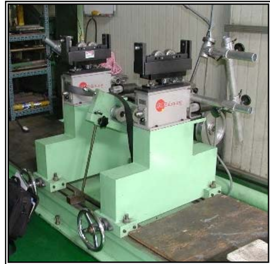
B50U Suspension & Roller Work Supports Mounted on Modified Pedestals
